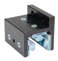
FATH 3-slot single-flange linear bearing, black, 63 x 80 x 67mm, aluminum/die-cast zinc/polyoxymethylene (POM), slot size 8. For use with all 1.5in profile T-slotted rails. Manufacturer part number: 093SF381S.
