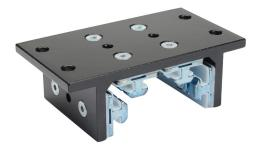
FATH 4-slot double-flange linear bearing, black, 143 x 80 x 48mm, aluminum/die-cast zinc/polyoxymethylene (POM), slot size 8. For use with all 3in profile T-slotted rails. Manufacturer part number: 093DF761S.
