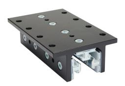
FATH 3-slot double-flange linear bearing, black, 103 x 160 x 48mm, aluminum/die-cast zinc/polyoxymethylene (POM), slot size 8. For use with all 1.5in profile T-slotted rails. Manufacturer part number: 093DF382S.
