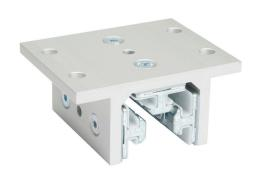
FATH 3-slot double-flange linear bearing, silver, 103 x 80 x 48mm, aluminum/die-cast zinc/polyoxymethylene (POM), slot size 8. For use with all 1.5in profile T-slotted rails. Manufacturer part number: 093DF381.
