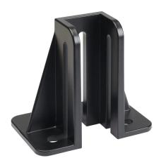
FATH foot console, black, 1.5 x 1.5in, die-cast aluminum, slot size 8. For use with all 1.5in profile T-slotted rails. Manufacturer part number: 098G38L85128AS.
