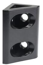
FATH wide gusseted inside corner bracket, black, 90-degree, 4 holes, aluminum, slot size 8. For use with all 1.5in and 3in profile T-slotted rails. Manufacturer part number: 093WD8384N08S.
