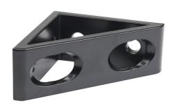
FATH tall gusseted inside corner bracket, black, 90-degree, 4 holes, aluminum, slot size 8. For use with all 1.5in and 3in profile T-slotted rails. Manufacturer part number: 093W8383N08S.
