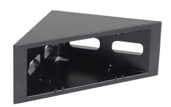
FATH inside corner bracket, black, 90-degree, 4 holes, die-cast zinc, slot size 8. For use with all 1.5in, 3in, 40mm, and 80mm profile T-slotted rails. Manufacturer part number: 093W802N08S.
