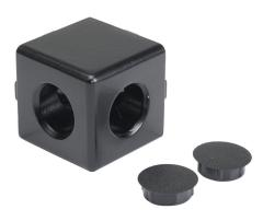
FATH 2D cube connector, black, 1.5 x 1.5 x 1.5in, die-cast aluminum, slot size 8. For use with all 1.5in and 3in profile T-slotted rails. (2) plastic cover caps included. Manufacturer part number: 093WW381N08S.
