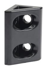
FATH wide gusseted inside corner bracket, black, 90-degree, 4 holes, aluminum, slot size 6. For use with all 1in and 2in profile T-slotted rails. Manufacturer part number: 093WD8104N06S.
