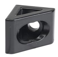
FATH gusseted inside corner bracket, black, 90-degree, 2 holes, aluminum, slot size 6. For use with all 1in and 2in profile T-slotted rails. Manufacturer part number: 093W8104N06S.
