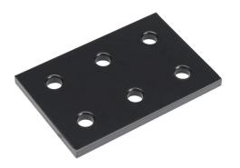
FATH rectangular flat plate, black, 6 holes, aluminum, slot size 6. For use with all 1in and 2in profile T-slotted rails. Manufacturer part number: 093EVD5176S.
