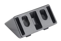
FATH angle connector, black, 45-degree, 1 x 2in, die-cast aluminum, slot size 6. For use with all 1in and 2in profile T-slotted rails. Manufacturer part number: 093WS51145N6,5S.
