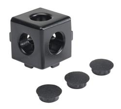
FATH 3D cube connector, black, 1 x 1 x 1in, die-cast aluminum, slot size 6. For use with all 1in and 2in profile T-slotted rails. (3) plastic cover caps included. Manufacturer part number: 093WW252N06S.
