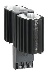
Stego enclosure heater, 75W heating capacity, PTC resistor heating element, 120-240 VAC/VDC operating voltage, 50/60 Hz, 35mm DIN rail or panel mount.
