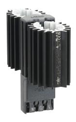
Stego enclosure heater, 75W heating capacity, PTC resistor heating element, 120-240 VAC/VDC operating voltage, 50/60 Hz, 35mm DIN rail or panel mount.
