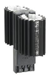
Stego enclosure heater, 60W heating capacity, PTC resistor heating element, 120-240 VAC/VDC operating voltage, 50/60 Hz, 35mm DIN rail or panel mount.
