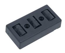
FATH roller element, black, thermoplastic polyurethane/nylon/steel, slot size 10. For use with all 45mm and 90mm profile T-slotted rails. Mounting hardware included. Manufacturer part number: 09309302.
