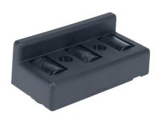
FATH roller element with guide, black, thermoplastic polyurethane/nylon/steel, slot size 10. For use with all 45mm and 90mm profile T-slotted rails. Mounting hardware included. Manufacturer part number: 09309304.
