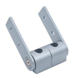
FATH 2-slot pivot joint, silver, 180-degree, die-cast zinc/die-cast aluminum/nylon, slot size 8. For use with all 80mm profile T-slotted rails. (4) slot keys included. Manufacturer part number: 093GV4080.
