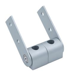
FATH 2-slot pivot joint, silver, 180-degree, die-cast zinc/die-cast aluminum/nylon, slot size 8. For use with all 60mm profile T-slotted rails. (4) slot keys included. Manufacturer part number: 093GV3060.
