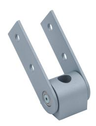
FATH 1-slot pivot joint, silver, 180-degree, die-cast zinc/die-cast aluminum/nylon, slot size 8. For use with all 30mm profile T-slotted rails. (2) slot keys included. Manufacturer part number: 093GV30.
