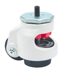
FATH leveling caster, off-white, M12-1.75, die-cast aluminum/ steel/nylon/rubber, slot size 6/8/10. For use with all 1.5in, 2in, 3in, 60mm, 80mm and 90mm profile T-slotted rails. Mounting hardware included.
