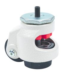
FATH leveling caster, off-white, M12-1.75, die-cast aluminum/ steel/nylon/rubber, slot size 6/8/10. For use with all 1.5in, 2in, 3in, 60mm, 80mm and 90mm profile T-slotted rails. Mounting hardware included.
