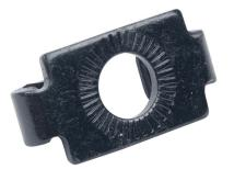
FATH screw connector, gloss black, zinc plated steel, slot size 8. Package of 10. For use with 30 x 30mm profile T-slotted rails. Manufacturer part number: 092039S04.
