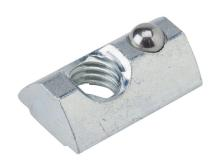
FATH roll-in nut, silver, M8-1.25, zinc plated steel, slot size 8. Package of 10. For use with all 1.5in, 3in, 40mm and 80mm profile T-slotted rails. Manufacturer part number: 096338.
