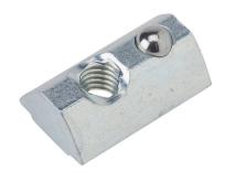
FATH roll-in nut, silver, M6-1.0, zinc plated steel, slot size 8. Package of 10. For use with all 1.5in, 3in, 40mm and 80mm profile T-slotted rails. Manufacturer part number: 096336.
