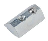
FATH roll-in nut, silver, M4-0.7, zinc plated steel, slot size 8. Package of 10. For use with all 1.5in, 3in, 40mm and 80mm profile T-slotted rails. Manufacturer part number: 096334.
