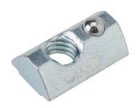
FATH roll-in nut, silver, 5/16-18 UNC, zinc plated steel, slot size 8. Package of 10. For use with all 1.5in, 3in, 40mm and 80mm profile T-slotted rails. Manufacturer part number: 09633U5/16.
