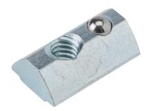
FATH roll-in nut, silver, 1/4-20 UNC, zinc plated steel, slot size 8. Package of 10. For use with all 1.5in, 3in, 40mm and 80mm profile T-slotted rails. Manufacturer part number: 09633U1/4.
