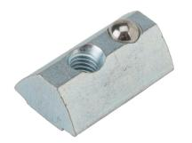
FATH roll-in nut, silver, 10-32 UNF, zinc plated steel, slot size 8. Package of 10. For use with all 1.5in, 3in, 40mm and 80mm profile T-slotted rails. Manufacturer part number: 09633U10-32.
