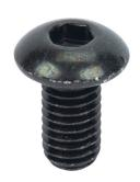
FATH button head socket cap screw, black, 8-32 UNF x 3/8in, zinc plated steel, slot size 6/8/10. Package of 10. For use with all T-slotted rails. Manufacturer part number: 4ISO7380U8-32.38M.
