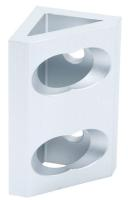
FATH wide gusseted inside corner bracket, silver, 90-degree, 4 holes, anodized aluminum, slot size 8. For use with all 60mm profile T-slotted rails. Manufacturer part number: 093WD8303N08.
