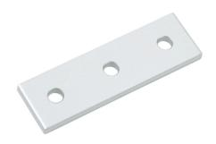
FATH straight flat plate, silver, 3 holes, anodized aluminum, slot size 8. For use with all 30mm and 60mm profile T-slotted rails. Manufacturer part number: 093VA3090.
