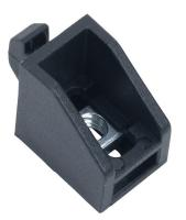
FATH panel uni-block, black, nylon, slot size 8. Package of 10. For use with all 1.5in, 3in, 40mm and 80mm profile T-slotted rails. Manufacturer part number: 094035U1/4.
