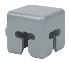
FATH clamp profile connector, silver, die-cast zinc, slot size 8. For use with 40 x 40mm profile T-slotted rails. (2) screws included. Requires FATH 162976 mounting element. Manufacturer part number: 093WWC401N08.
