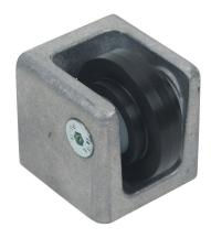
FATH sliding door guide, silver/black, die-cast aluminum/nylon, slot size 8. For use with all 40mm and 80mm profile T-slotted rails. Manufacturer part number: 093095.
