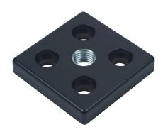
FATH transport/base plate, black, 90 x 90mm, M20-2.5, die-cast zinc, slot size 10. For use with 90 x 90mm T-slotted rails. Mounting hardware included. Manufacturer part number: 093T90902012S.
