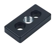
FATH transport/base plate, black, 45 x 90mm, M20-2.5, die-cast zinc, slot size 10. For use with 45 x 90mm T-slotted rails. Mounting hardware included. Manufacturer part number: 093T45902012S.
