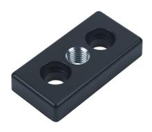
FATH transport/base plate, black, 45 x 90mm, M16-2.0, die-cast zinc, slot size 10. For use with 45 x 90mm T-slotted rails. Mounting hardware included. Manufacturer part number: 093T45901612S.
