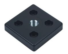
FATH transport/base plate, black, 80 x 80mm, M16-2.0, die-cast zinc, slot size 8. For use with 80 x 80mm T-slotted rails. Mounting hardware included. Manufacturer part number: 093T80801608S.
