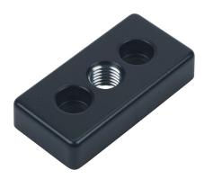
FATH transport/base plate, black, 40 x 80mm, M16-2.0, die-cast zinc, slot size 8. For use with 40 x 80mm T-slotted rails. Mounting hardware included. Manufacturer part number: 093T40801608S.
