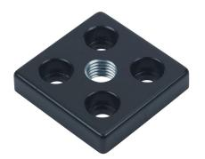
FATH transport/base plate, black, 60 x 60mm, M16-2.0, die-cast zinc, slot size 8. For use with 60 x 60mm T-slotted rails. Mounting hardware included. Manufacturer part number: 093T60601608S.
