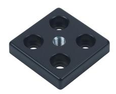
FATH transport/base plate, black,  $60 \times 60$ mm, M10-1.5, die-cast zinc, slot size 8. For use with  $60 \times 60$ mm T-slotted rails. Mounting hardware included. Manufacturer part number: 093T60601008S.
