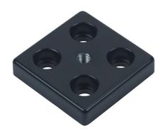
FATH transport/base plate, black,  $60 \times 60$ mm, M8-1.25, die-cast zinc, slot size 8. For use with  $60 \times 60$ mm T-slotted rails. Mounting hardware included. Manufacturer part number: 093T60600808S.
