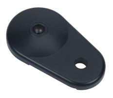
FATH extended swivel base, black, 80mm, die-cast zinc, ball joint size 15. For use with all T-slotted rails. Requires ball joint size 15 swivel foot threaded rod. Manufacturer part number: 098DA080ZSG.
