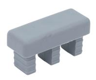
FATH cover cap, gray, 8 x 40 x 16mm, thermoplastic rubber, slot size 8. Package of 10. For use with FATH 162929 side protection profile and 162930 corner protection profile. Manufacturer part number: 091385.
