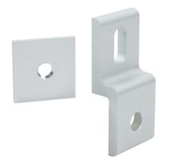
FATH panel holder, silver, anodized aluminum, slot size 8. For use with all 30mm and 60mm profile T-slotted rails. Backing plate included. Manufacturer part number: 093P30LN.
