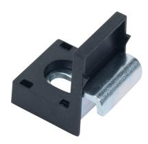
FATH top angle clamp, black, 90-degree, nylon/steel, slot size 8. For use with all 40mm and 80mm profile T-slotted rails. Mounting hardware included. Manufacturer part number: 093WT401N08S.
