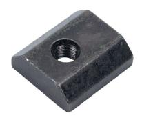
FATH slide-in nut, black, 10-32 UNF, zinc plated steel, slot size 8. Package of 10. For use with all 1.5in, 3in, 40mm and 80mm profile T-slotted rails. Manufacturer part number: 096ST15U10-32.
