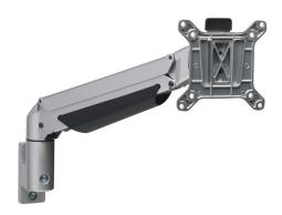
FATH 4-axis mounting support, silver, 438 x 100 x 236mm, diecast aluminum/plastic/steel, slot size 8/10. For use with all 1.5in, 3in, 40mm, 45mm, 80mm and 90mm profile T-slotted rails. Mounting hardware included. Manufacturer part number: 6MHM75100S40.
