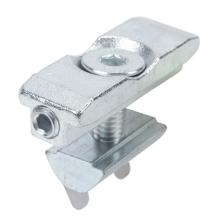
FATH direct connector, silver, steel, slot size 8. For use with all 1.5in, 3in, 40mm and 80mm profile T-slotted rails. Manufacturer part number: 099DC084040N08.
